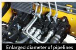
Enlarged diameter of pipelines
